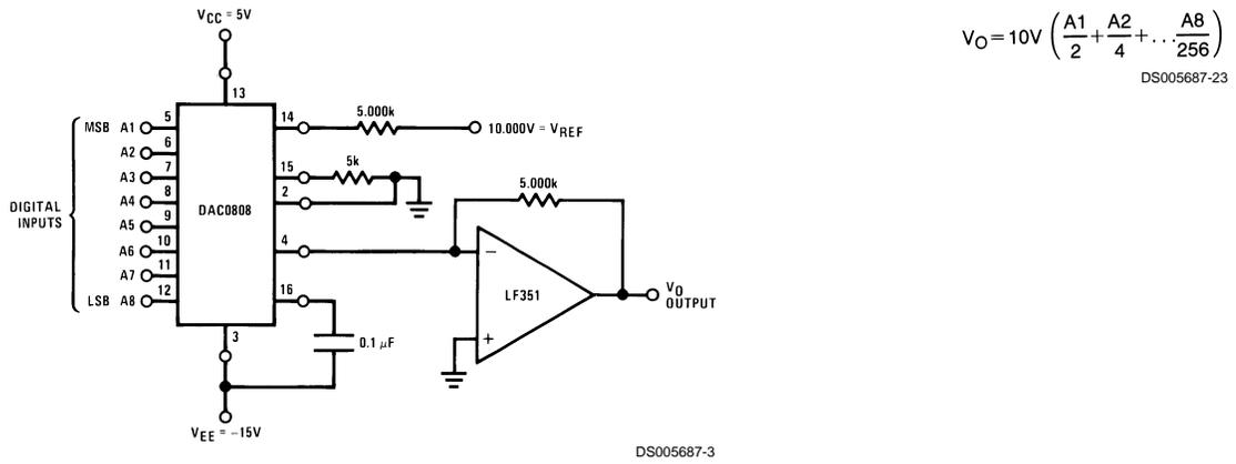
FIGURE 1. +10V Output Digital to Analog Converter (Note 8)
