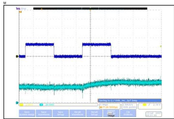
**FIGURE 2-45:** 100 k $\Omega$  – Power-Up Wiper Response Time (1  $\mu\text{s}/\text{Div}$ ).
