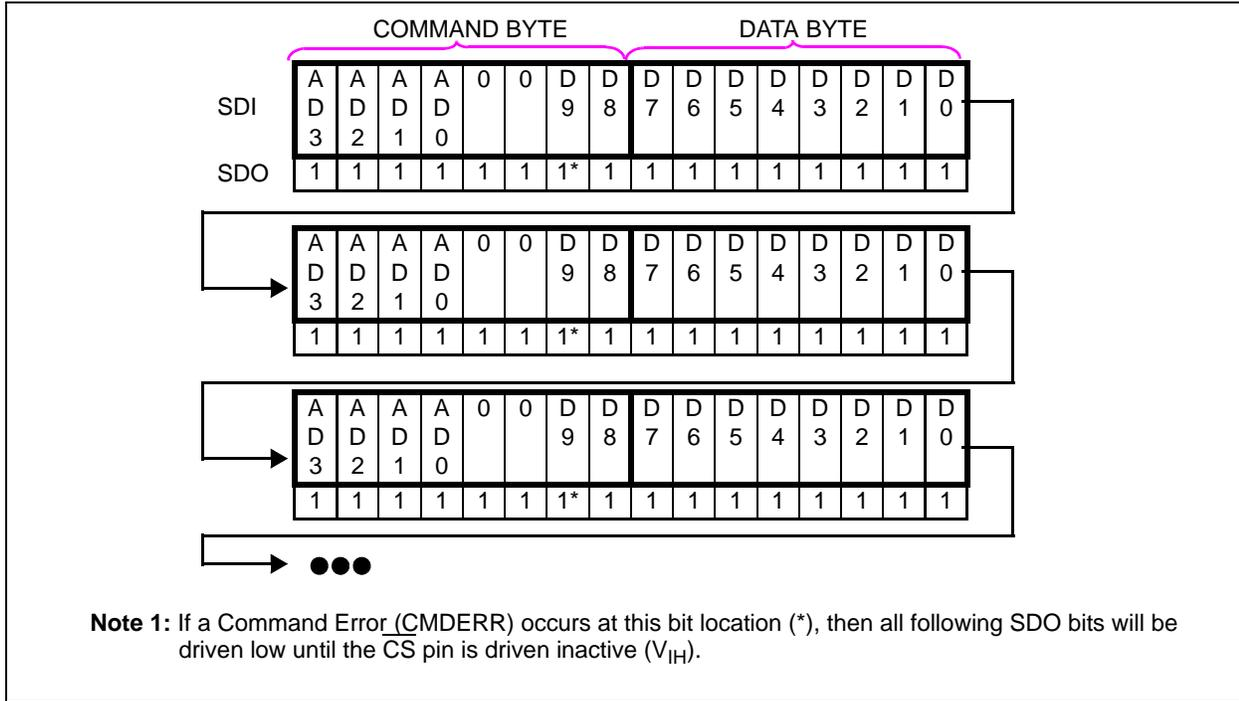
**FIGURE 7-3:** Continuous Write sequence (Volatile Memory only).
