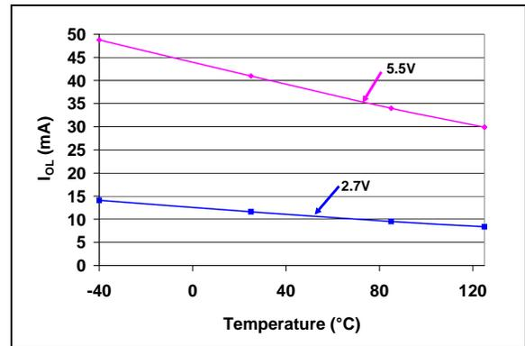
**FIGURE 2-54:**  $I_{OL}$  (SDO) vs.  $V_{DD}$  and Temperature.
