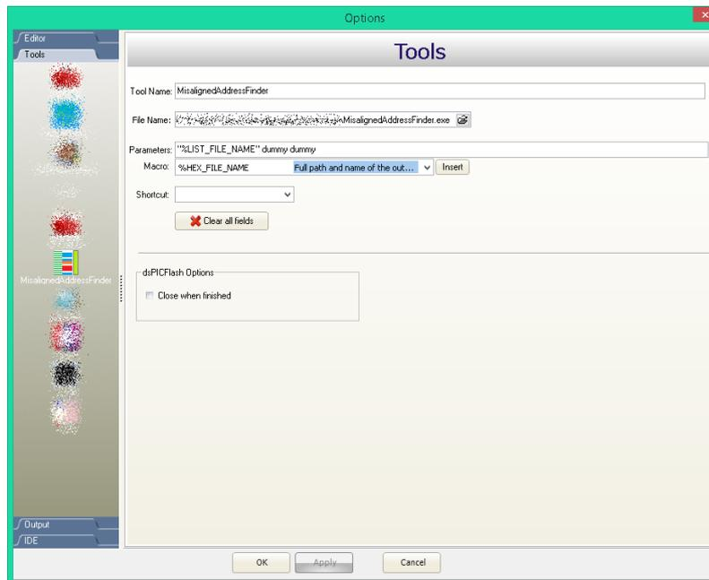
As command line parameters, users should fill in: **"%LIST\_FILE\_NAME" dummy**
