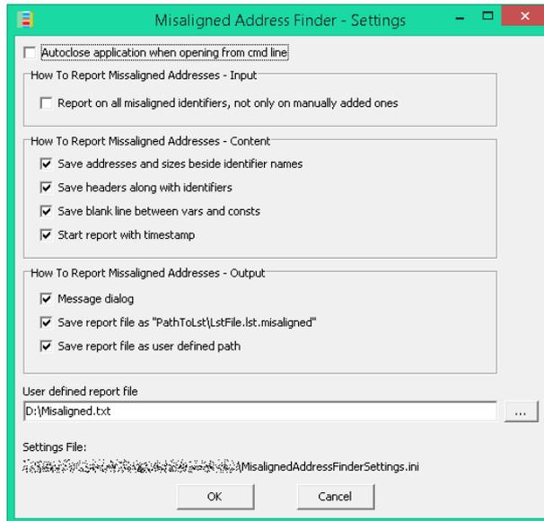
Using the [Settings](#) button, the Settings window will be displayed, allowing users to configure various reporting options. When the [Autoclose application when opening from cmd line](#) checkbox is checked, the application closes automatically after generating the report. An exception to this is when the application is started without a `lst` file, sent as command line argument. Also, when the report is generated from the pop-up menu of the list of `lst` files, the application will not close.
