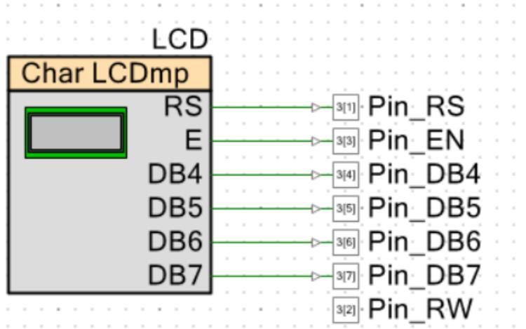
All lcd pines lcd are configured as outputs
