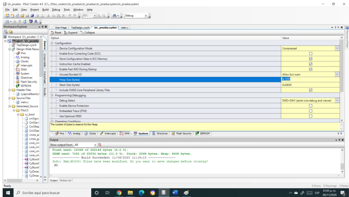
8) build before writing the code so that the necessary files are added to the project
