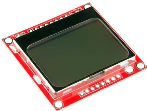
Though PCD8544 supports SPI communication method, here in this example bit-banging method is used. Thus, we can realize it being driven by software SPI instead of hardware-based SPI.
