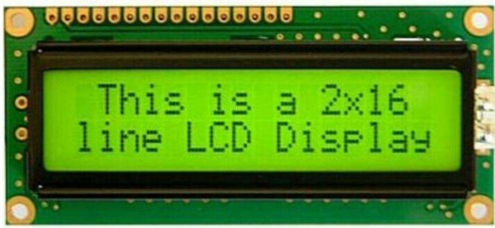
Be sure to use 3.3V compatible LCD because most of them don't operate at 3.3V power level. Most of the LCD are designed for 5V operation. It is okay to use 5V power supply for powering LCD if there is no other option. LCDs accept 0V - 3.3V logic level. However, there should be no way with which a 5V power supply/device can get connected with MSP430's 3.3V power bus.
