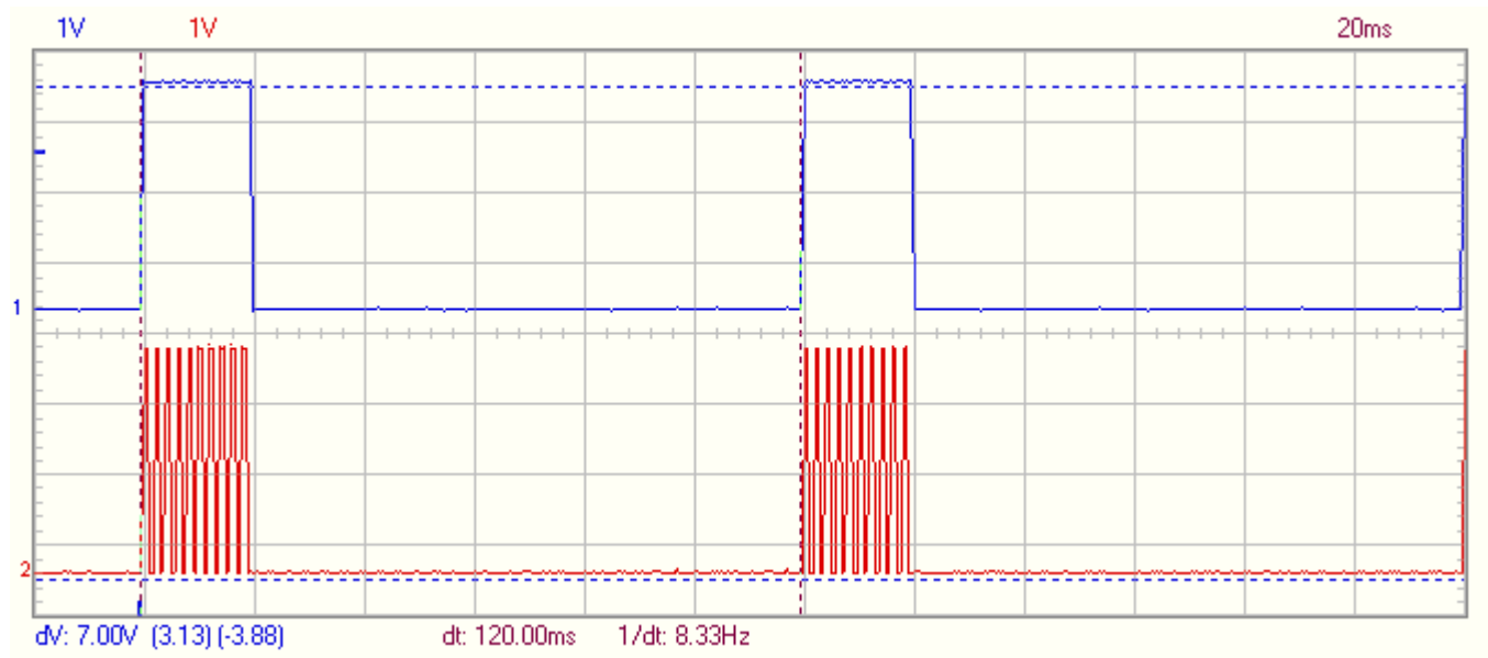
Figure 1: DelayedOut_bit (blue) and OscOut_bit (red)
