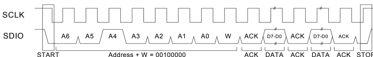
**Figure 6. 2-Wire Control Interface Write Timing Diagram**
