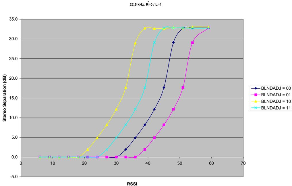
**Figure 10. Stereo Separation**
