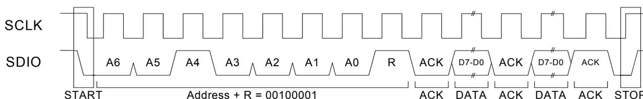
**Figure 7. 2-Wire Control Interface Read Timing Diagram**
