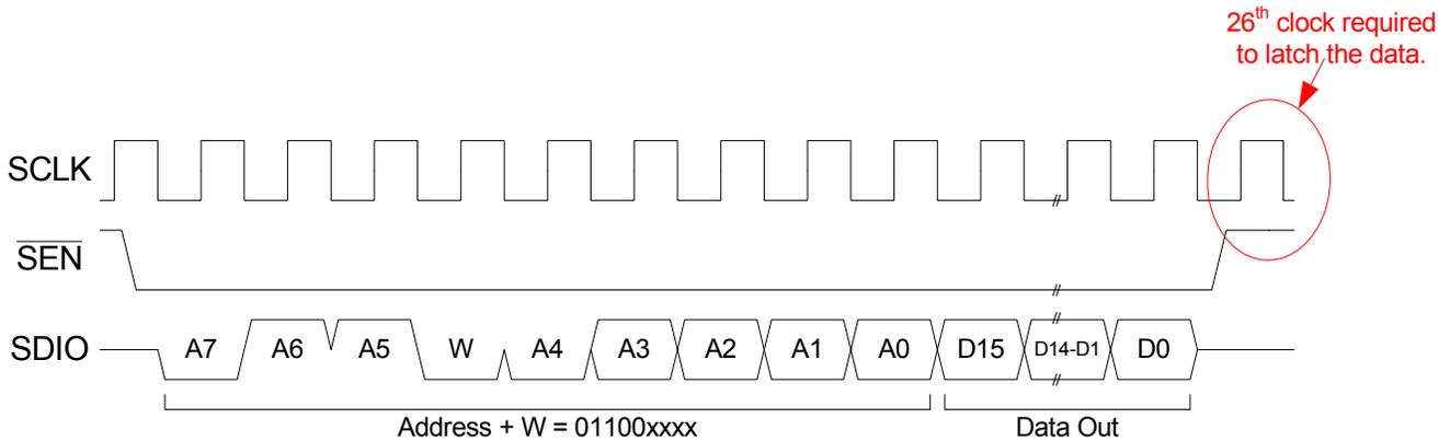
**Figure 4. 3-Wire Control Interface Write Timing Diagram**
