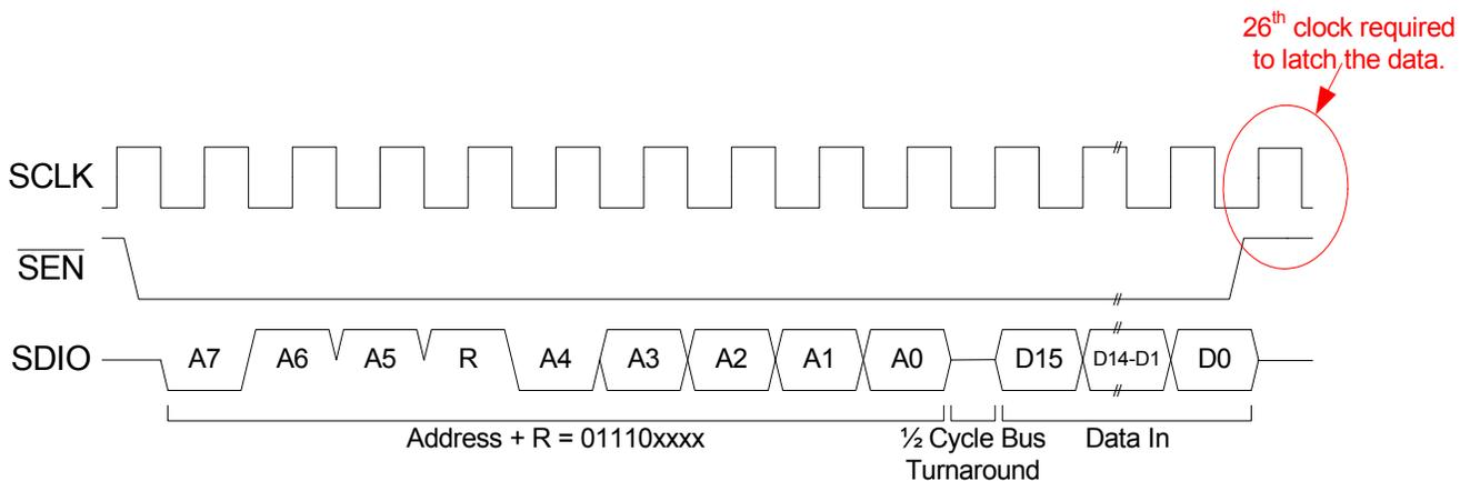
**Figure 5. 3-Wire Control Interface Read Timing Diagram**
