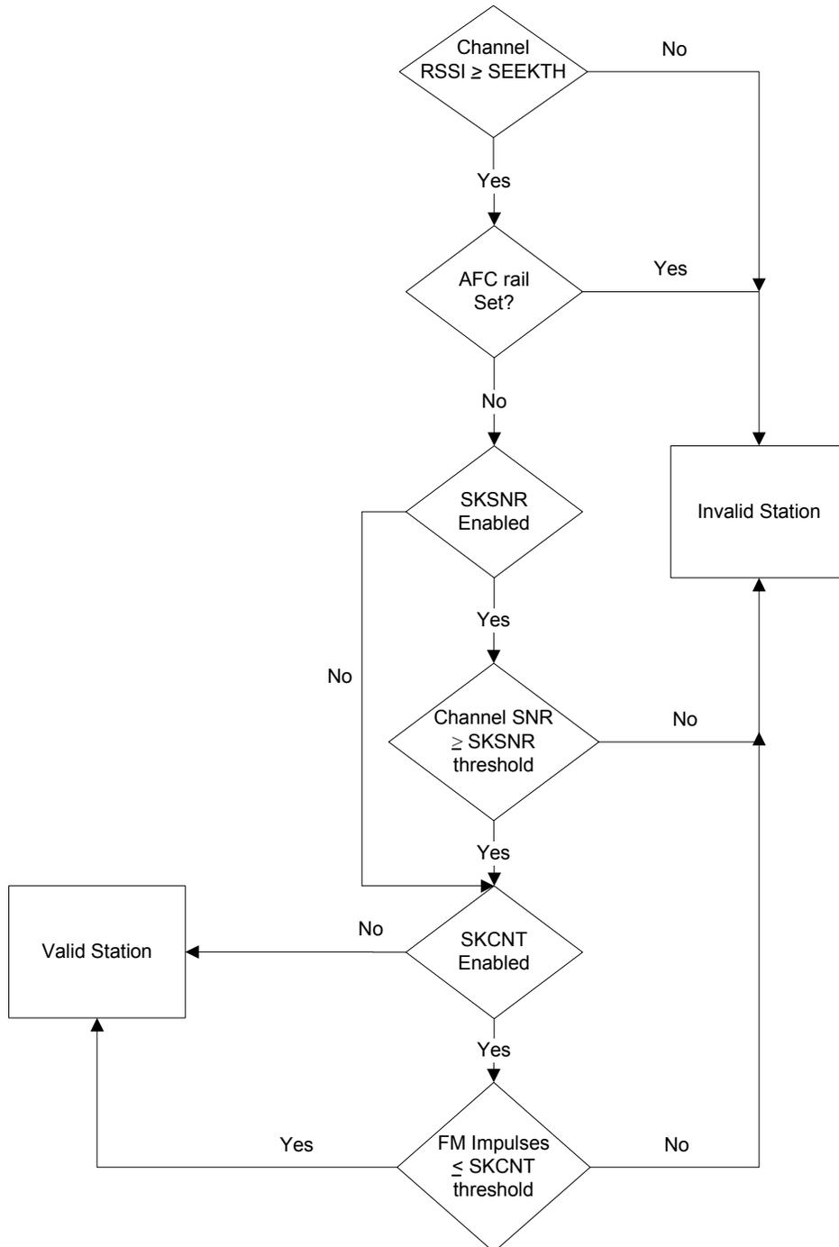
**Figure 18. Seek Algorithm Flowchart**
