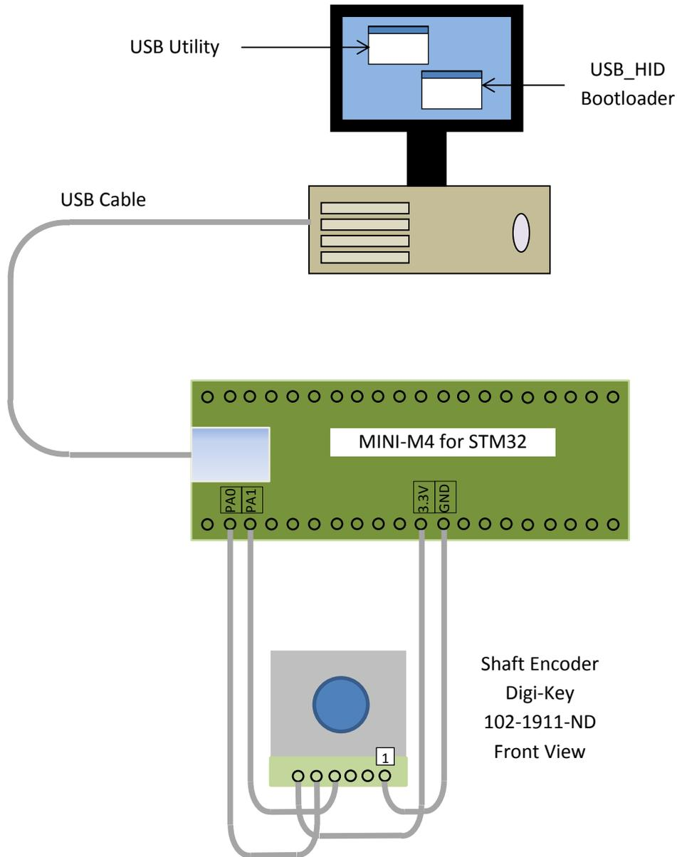
Although the shaft encoder shown is rated for 5V DC, it seems to work well on 3.3V DC. The connection pads on the shaft encoder are very small. It requires a skilful and delicate soldering technique to connect the wires. A flat cable is recommended.
