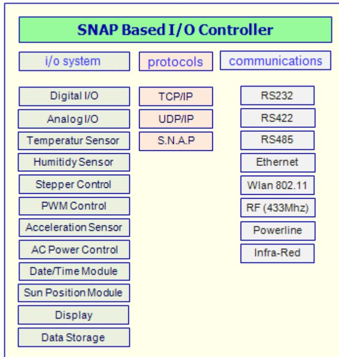
Each i/o module has separate data and control structures. The ctrl and data structures are essentially used within the PIC micro controller environment as well as in any control application (ie) under 'Window O/S' or web driven by using the same ctrl and data structures in a 'python' module. Changes in application control and data structures are reflected in the various i/o structures associated with an i/o module.
